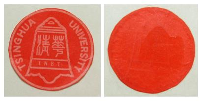
Drip-Disappear type: Daubed the Drip-Disappear type label with transparent liquid such as water or alcohol. The figure on the label will disappear until the evaporation of the liquid
